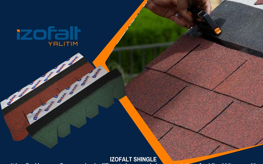
It is a final layer roofing covering in different shapes and sizes, consisting of oxidised bitumen with mineral stone particles on the upper surface, glass fibre preventing tearing and breaking in the middle part, and the lower surface is covered with a layer of rubber-mixed bitumen in order to adhere to the ground on which it is applied.
